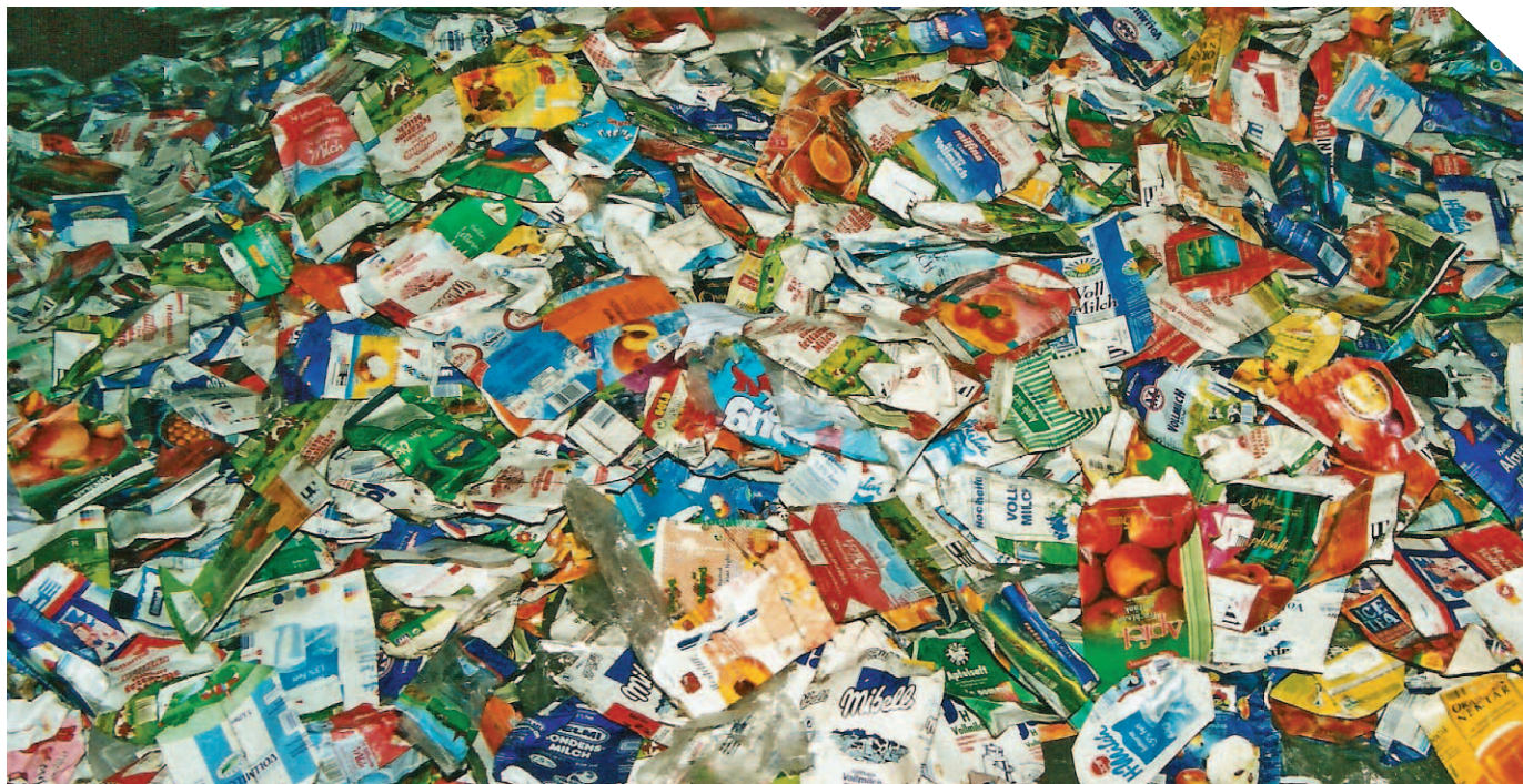
Storage silo full of drink cartons, automatically sorted by the CartonSort™ NIR optical sorting module.
