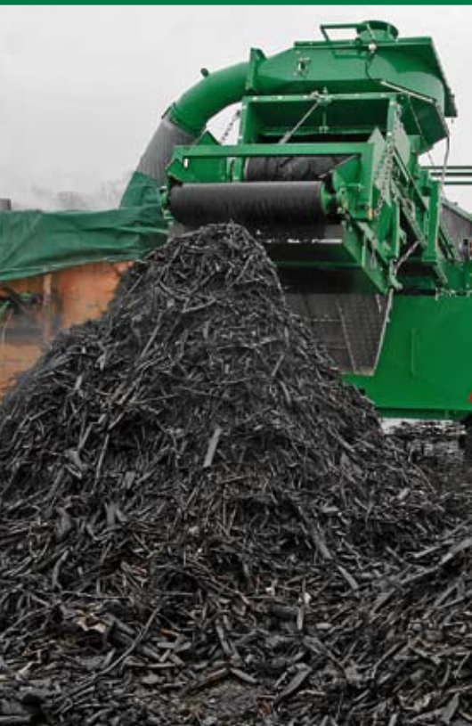
Screening residue from composting
